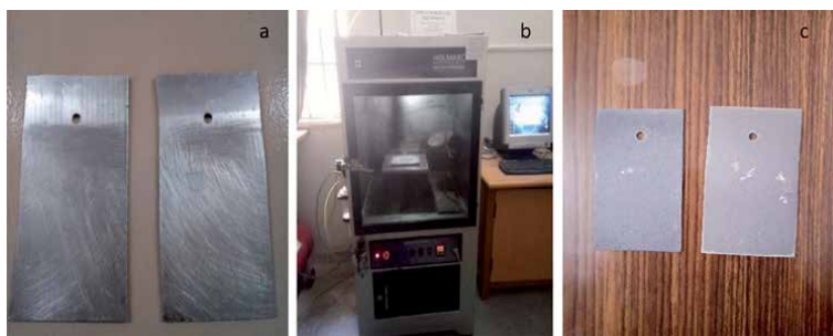
Figure 1. (a) Photograph of the pretreated zinc plate, (b) Coating on zinc in spray pyrolysis, (c) \text{TiO}_2/\text{Zn} .
