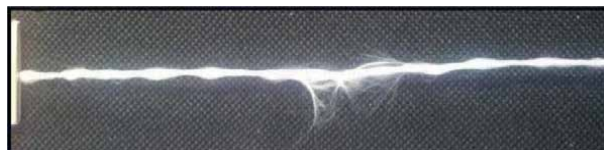
Figure 12. Yarn breaking strength testing [33].
