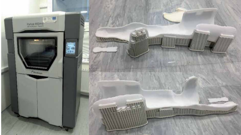
Figure 4. Fortus 450mc 3D printer (left) and an example of an orthoses manufactured by this machine (right).
