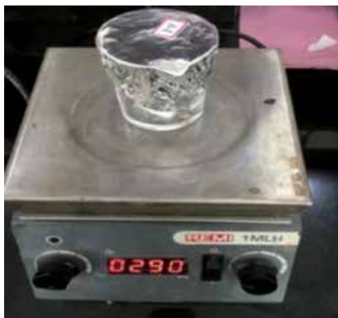
Figure 13. Actual setup of pure PMMA solution by magnetic stirrer and ultrasonication.
