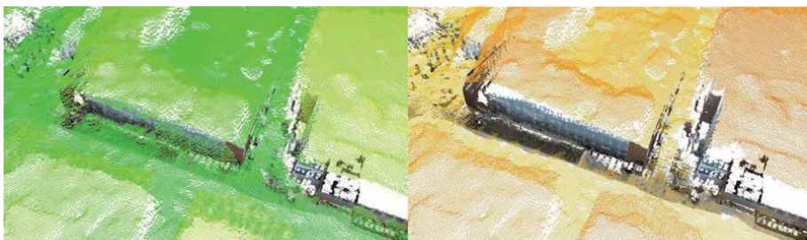
Figure 9. Co-registered cross-view point clouds are fused (left: before; right: after) by only keeping the high resolution results. Non-textured points are over-view satellite point clouds.
