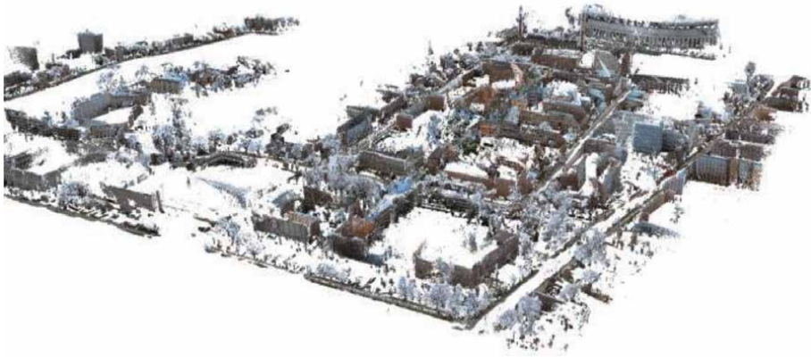
Figure 12. Dense reconstruction using our processing pipeline for two thirds of the campus region, totaling 7 billion color points.
