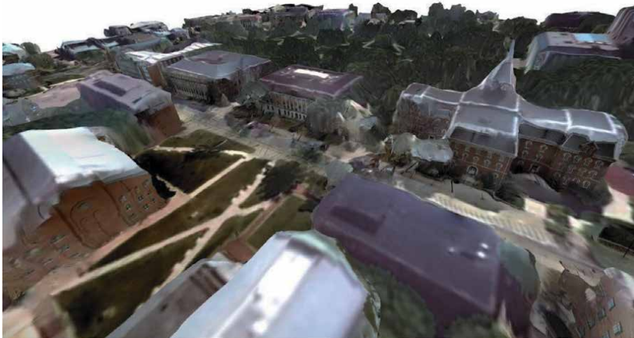
Figure 15. A screenshot of the generated textured mesh of the OSU campus area using our proposed pipeline, which includes information from the top-view and details on the facades.
