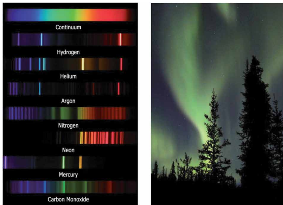
Figure 10. Emission spectra of some gases and aurora borealis.
