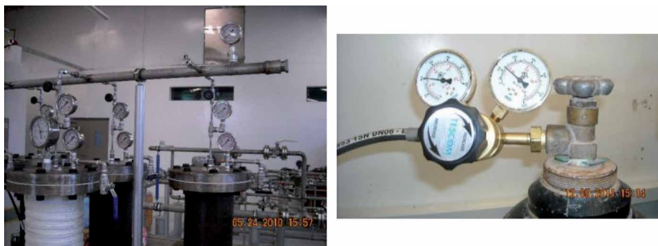
Figure 10. High-pressure manifold with connections to test units (left); pressure regulator to control high pressure flow into the test units (right).
