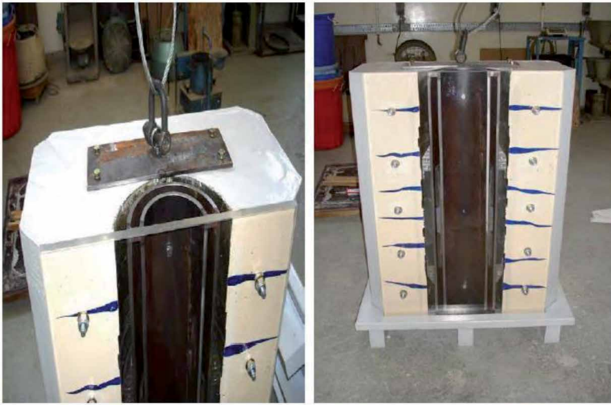
Figure 8. Fitting of the tubular in the concrete block, together with the lifting arrangement (left); fixing of the plexi-glass front wall (right).
