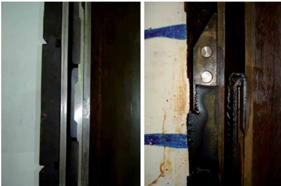
Figure 12. Elastomer seals before exposure to water (left), and after near-complete swelling of the outer packer (right); inner packer has only partially expanded.
