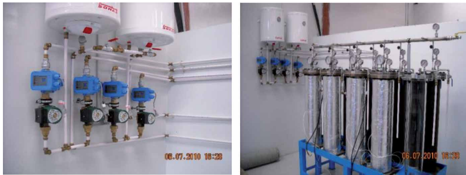
Figure 12. Ambient and hot water circulation system (left); complete assembly of the longevity test setup.
