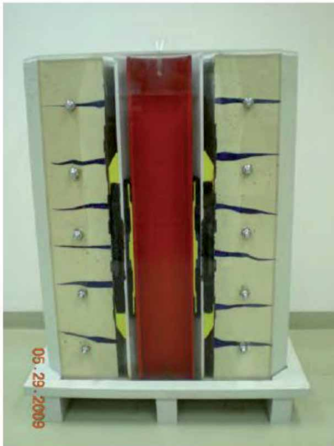
Figure 16. Experimental unit after one year of re-swell showing the swelling durability.
