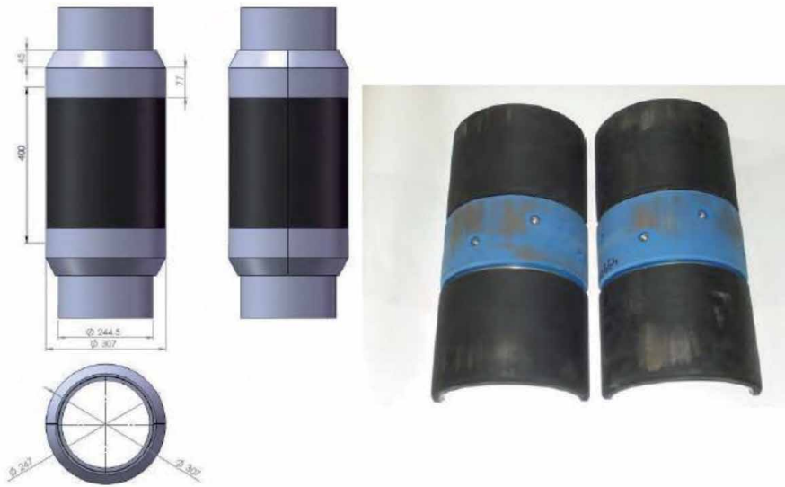
Figure 6. Dimensions and cut-away sections of the swell packer.
