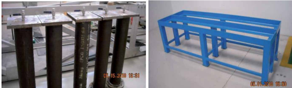
Figure 6. Fixing of drain valves to bottom plates (left); base frame to hold the test units (right).
