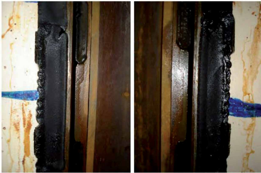
Figure 13. Near-complete swelling of the outer elastomer seals against cavities of varying diameter and roughness.
