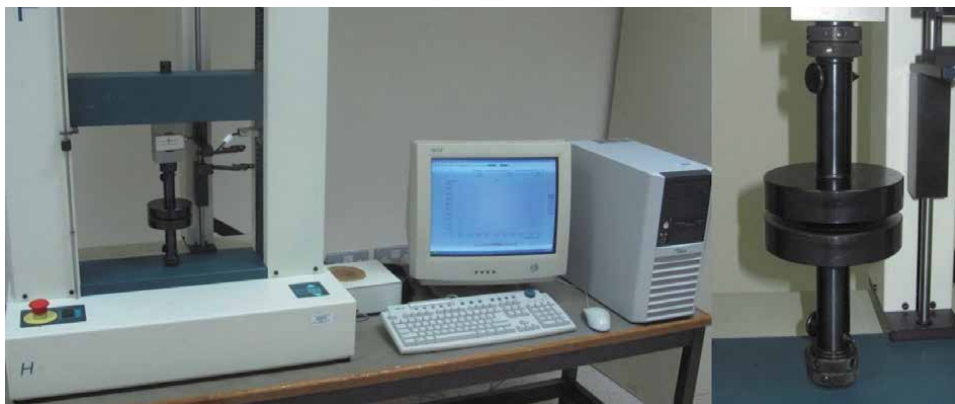
Figure 7. Setup for compression testing, using disc samples.
