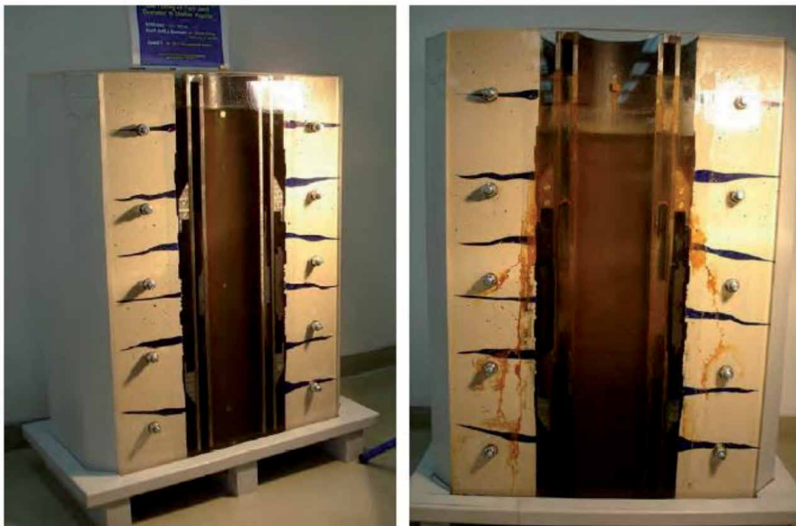
Figure 10. Assembled unit after initial water fill-up (left); rust stains after 8 days of water exposure (right).
