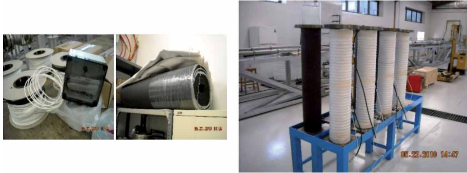
Figure 8. Thermal system components (left); winding of thermal blankets on casings (right).
