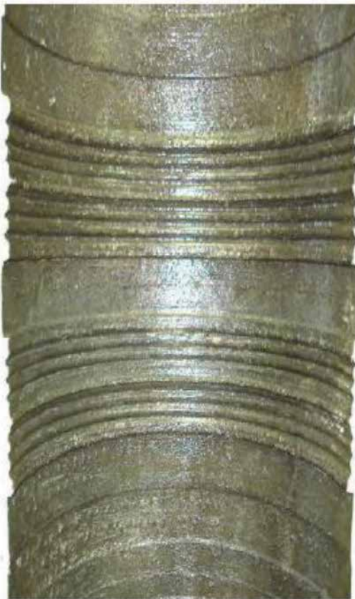
Figure 5. Close-up showing variation of diameter and roughness in the concrete half-block.
