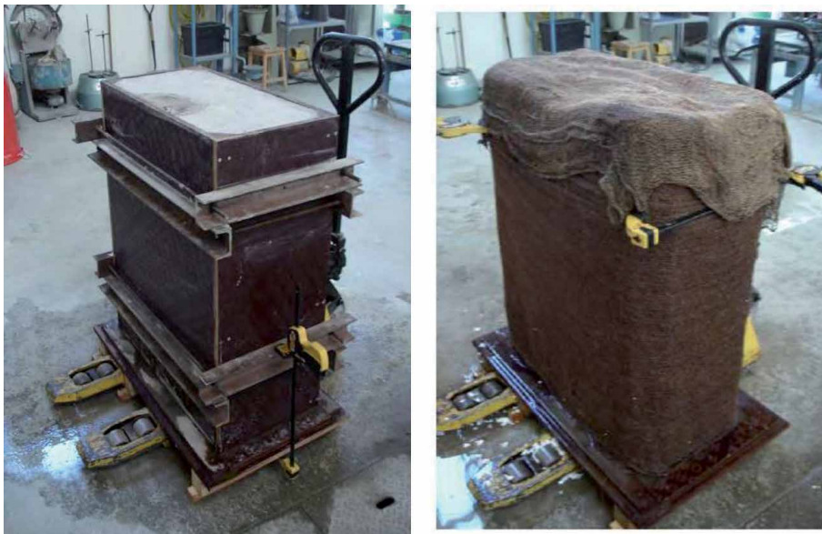
Figure 3. Concreting of the half-block with polystyrene half-cylinder carefully placed inside; and curing of the assembly.
