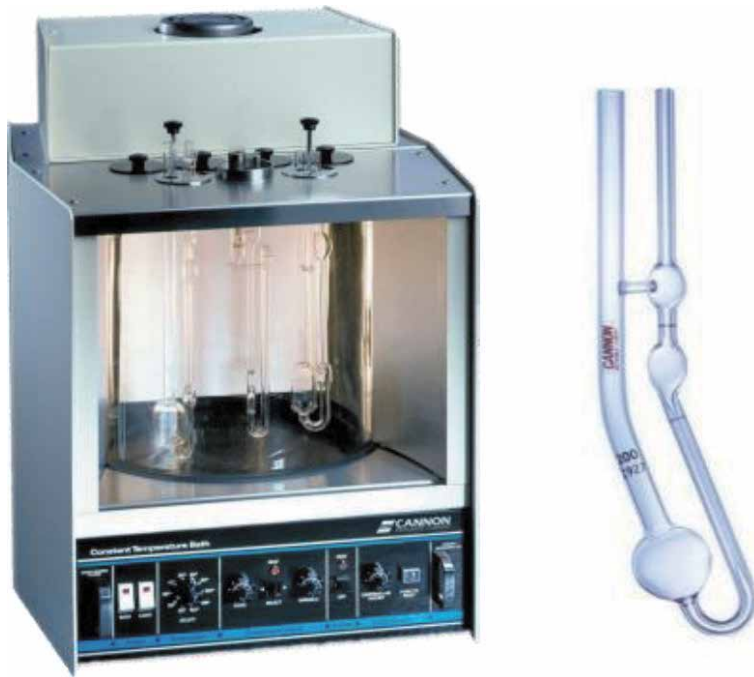
Figure 6. Cannon-Fenske apparatus used for viscosity measurement.
