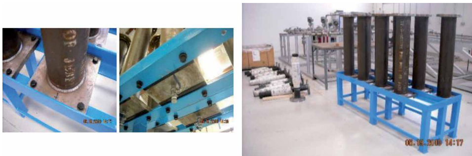
Figure 7. Fixing of casings to base frame (left); placement of packers inside casings (right).
