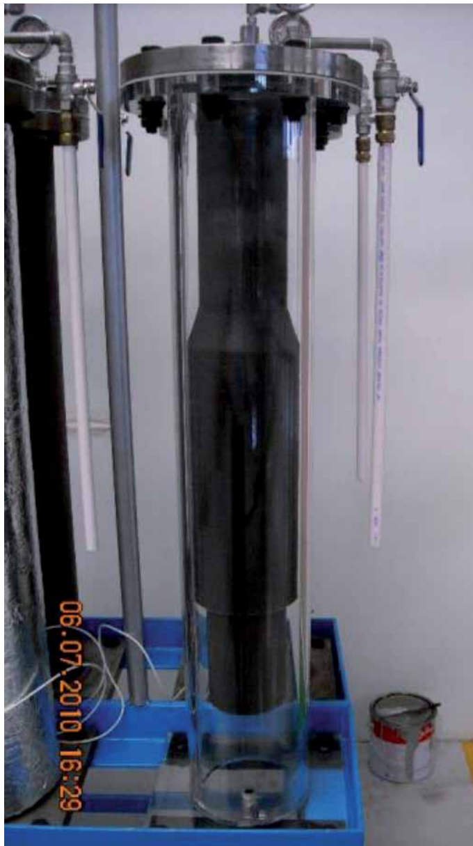
Figure 11. Perspex demonstration unit showing internal construction of other test units.
