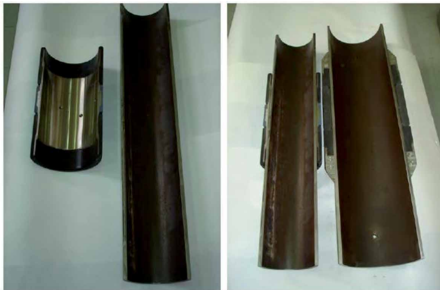
Figure 7. Half portions of inside swell packer and pipe (left); inside and outside swell packers fitted on respective pipes (right).
