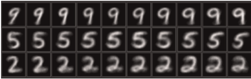
Figure 5. Sampled digits in continuous x, y values from the latent space interpolation. The conditioner of the vector changes only on the dimension that represents each class: 9, 5, and 2, respectively, top to bottom.
