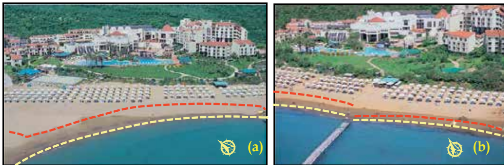
Fig. 8. Perissia Hotel Beach at Side; shoreline retreat due to erosion over the years, red line shows the shoreline position approximately in August, 2006 (a: view of the western part of the beach from sea, b: view of the eastern part of the beach from sea; pictures from 1999; Güler et al., 2008)
