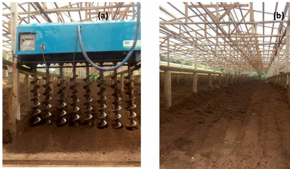
Figure 3. Mechanized composting system of swine effluents (a) [58], shaving bed after effluent injection and revolving (b) municipality of Concordia, SC.
