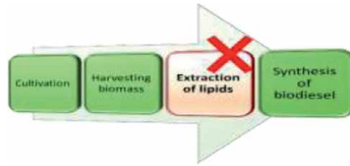
Figure 7. The “In situ” Transesterification process use of the raw material without the need to prioritize oil extraction.
