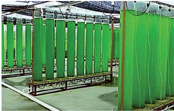
Figure 11. Vertical tubular photobioreactors for culturing microalgae [23].
