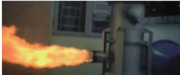
Figure 1. Gasification of oil-extracted cashew nut shell at Laboratory of Biofuel and Biomass Research, Ho chi Minh City University of Technology (HCMUT).
