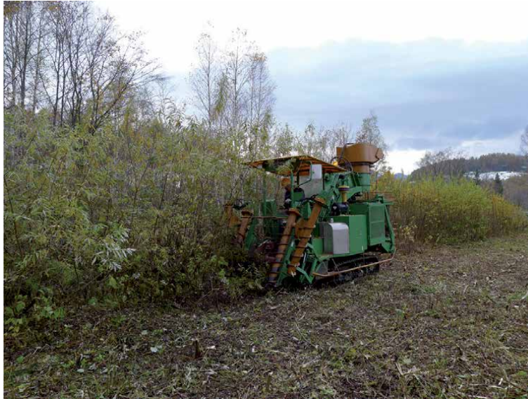
Figure 23. Experiment of harvesting willow trees using a sugarcane harvester.
