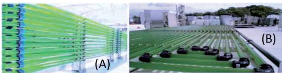
Figure 12. Horizontal tubular photobioreactor of different orientations [27]: (A) standing tubular bioreactor. The cultivation area occupied is less compared to the floor-type. (B) floor tubular reactor. This occupies a large cultivation area.
