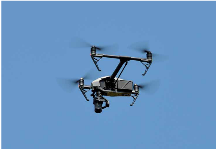
Figure 14. Four-rotor DJI INSPIRE 2 UAV equipped with Sentera Multispectral Double 4K camera used in this study.
