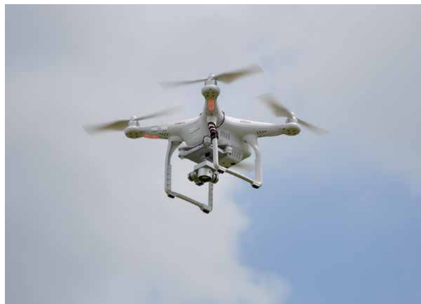
Figure 8. Four-rotor Phantom 2 Vision+ UAV equipped with a high-resolution digit RGB camera used in this study.
