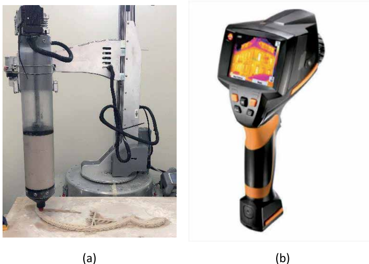
Figure 2. Tools used in this research: (a) Potterbot SLX-2 (Scara) printer; and (b) thermal imaging scanner 875-2i.
