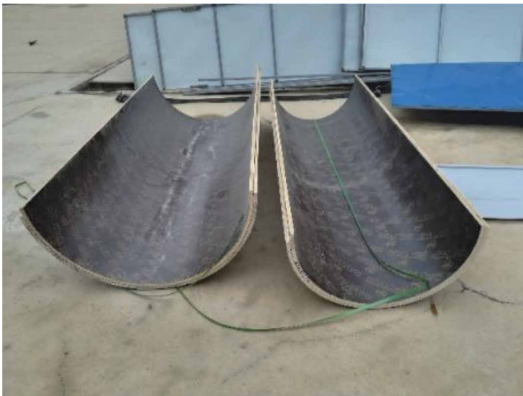
Figure 4. Molds for concrete casting.
