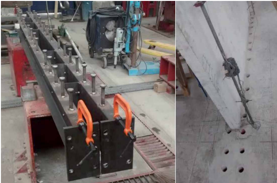
Figure 17. C-shaped steel channel with stud shear connectors (left), drills in the concrete slab.
