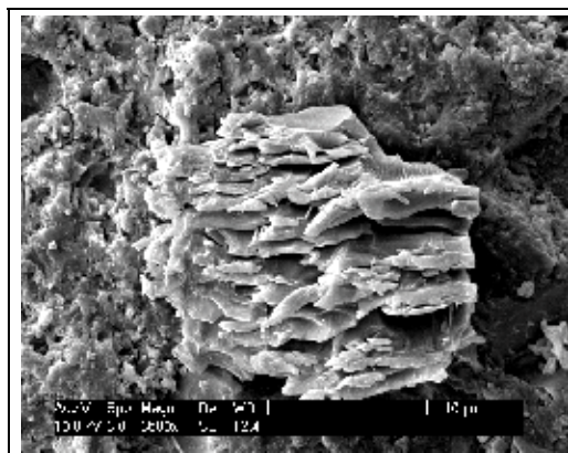
Fig. 15. Decomposition of aluminosilicate in a quartz rich matrix through high sintering
