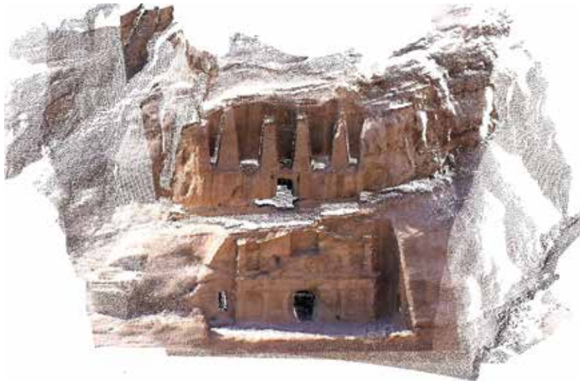
Fig. 2. 3D view of the four point clouds collected for the Obelisk Tomb and the Bab As-Siq Triclinium in Petra/Jordan.
