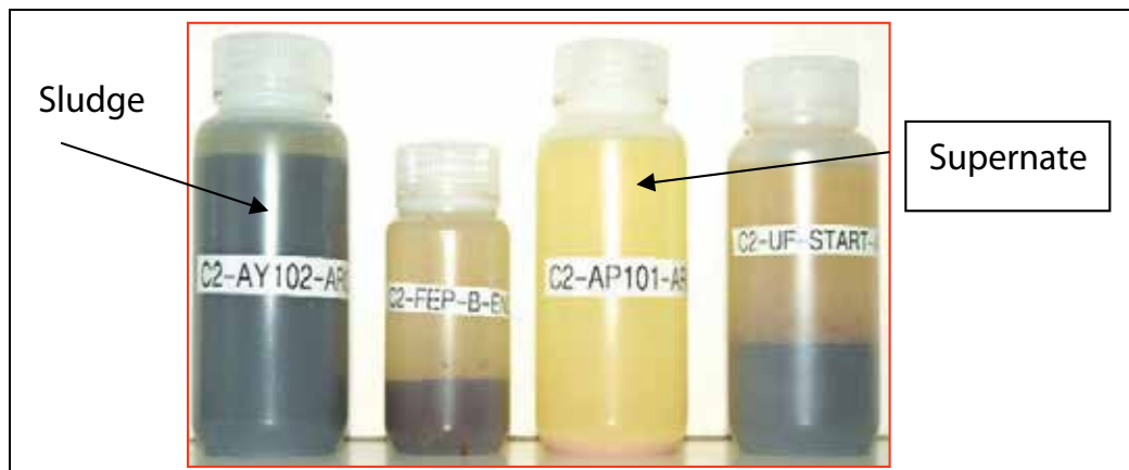
Fig. 2. Non-radioactive chemical simulants of the nuclear waste containing sludge and salt supernates (Note the opaque nature of sludges that form concentrated (5 - 50%) Fe/Al slurries limiting traditional light microscopy methods)
