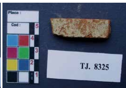
Fig. 4. Salt recrystallization on the surface through capillary effect of high porosity ceramics.
