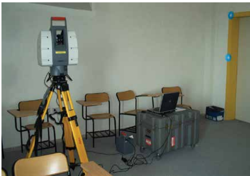
Fig. 2.2. Terrestrial Laser Scanner Used In This Application and Its Components
