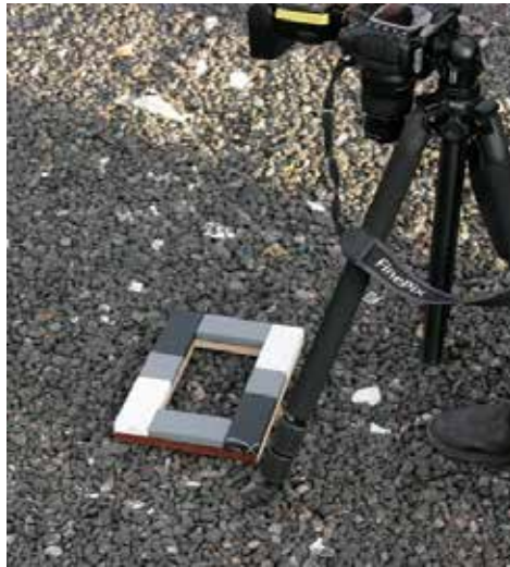
Fig. 6. Using digital camera and calibration frame to measure sample areas in Espoonlahti, Finland.
