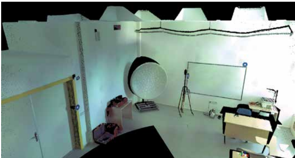
Fig. 1.1. Sample Point Cloud Data from TLS
