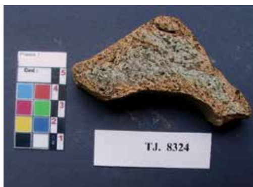
Fig. 1. Ceramic with different colors in the matrix as a function of uncontrolled firing.
