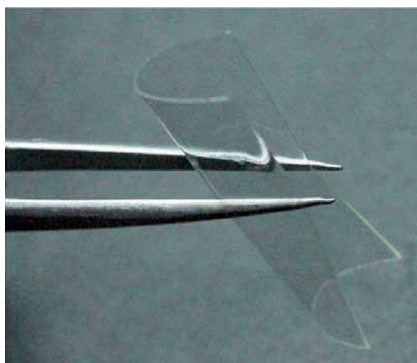
Figure 4. Flexible polymeric film (Adopted from [34]; OSA Publishing, 2018).
