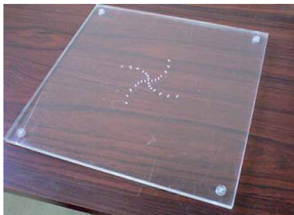
Figure 7. Central slabs of Perspex phantoms used for the experimental determination of radial dose function values.
