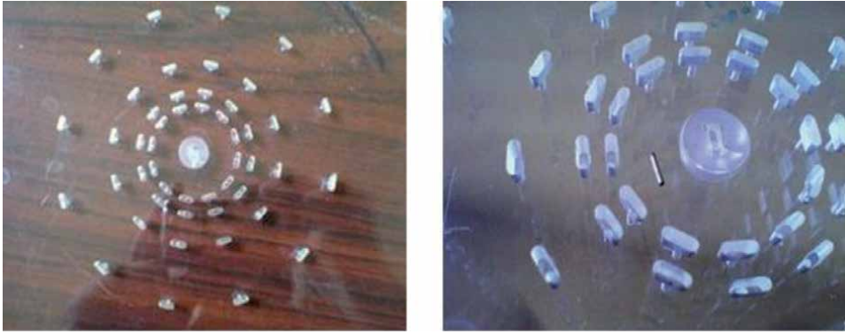
Figure 8. Central slabs of Perspex phantoms used for the experimental determination of anisotropy function values.
