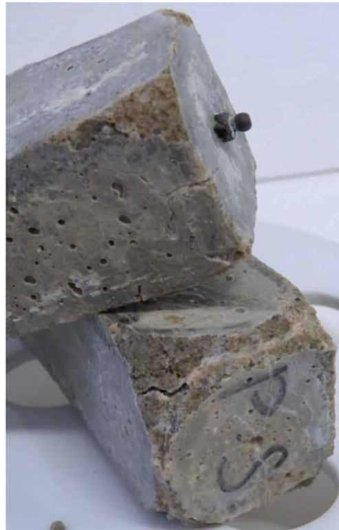
Figure 4. View on the disturbed surface of PC-mortar exposed for 5 years in 5% sodium sulfate solution.
