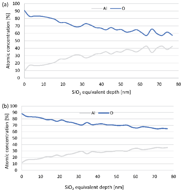
Figure 4. Depth profile analysis of Al 1050 (a) room temperature (b) 400°C annealed.
