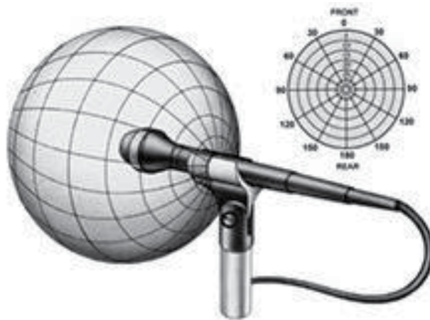
Figure 3. Omnidirectional pickup pattern in a microphone.
