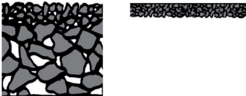
Figure 18. Two-layer porous asphalt (on the left) and a thin surface layer of asphalt (on the right) [1].
