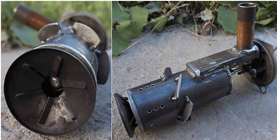
Figure 13. Flame head of liquid fuel burner with nozzle for co-combustion of gaseous fuel.
