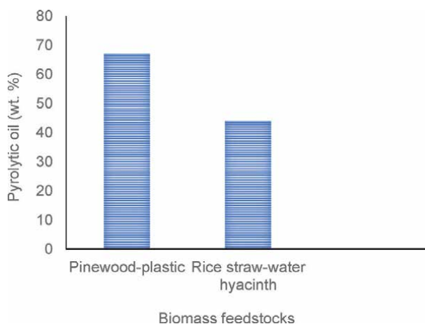
Figure 7. Pyrolytic oil generation from biomass co-pyrolysis process at 400 °C [9, 42].
