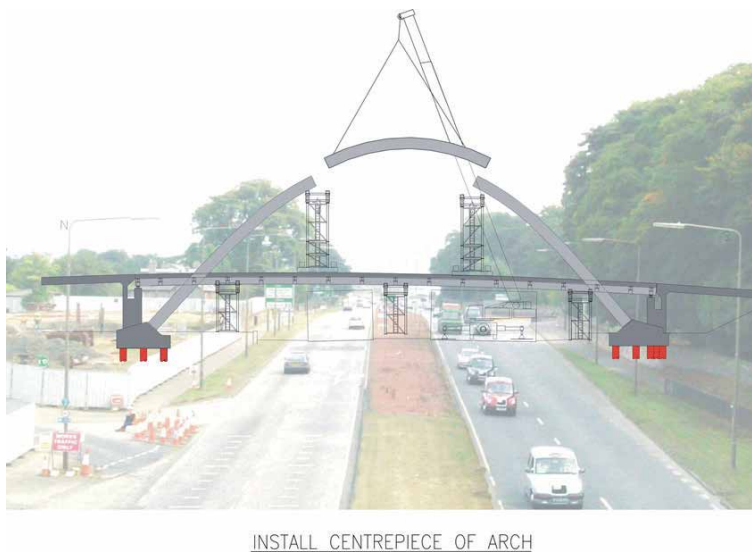
Figure 15. Erection sequence of the bridge, trestle.
