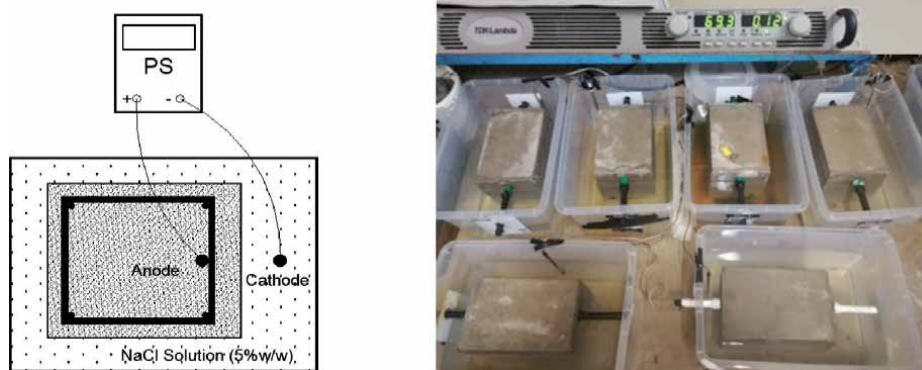
Figure 3. Simplified procedure of accelerated electro-corrosion (left) - accelerated corrosion experiments on RC specimens via inducing current (right).
