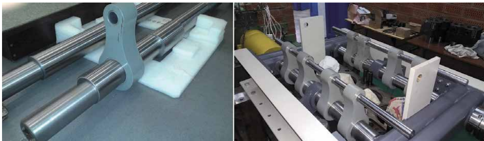
Figure 11. Connecting yokes mounted with the eccentric shafts.
