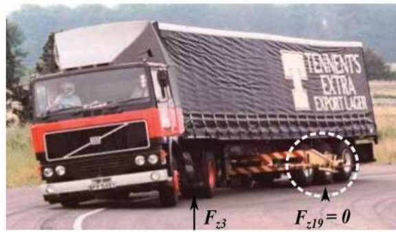
Figure 32. Dynamic rollover test. Source: Adapted of Cabral [33].
