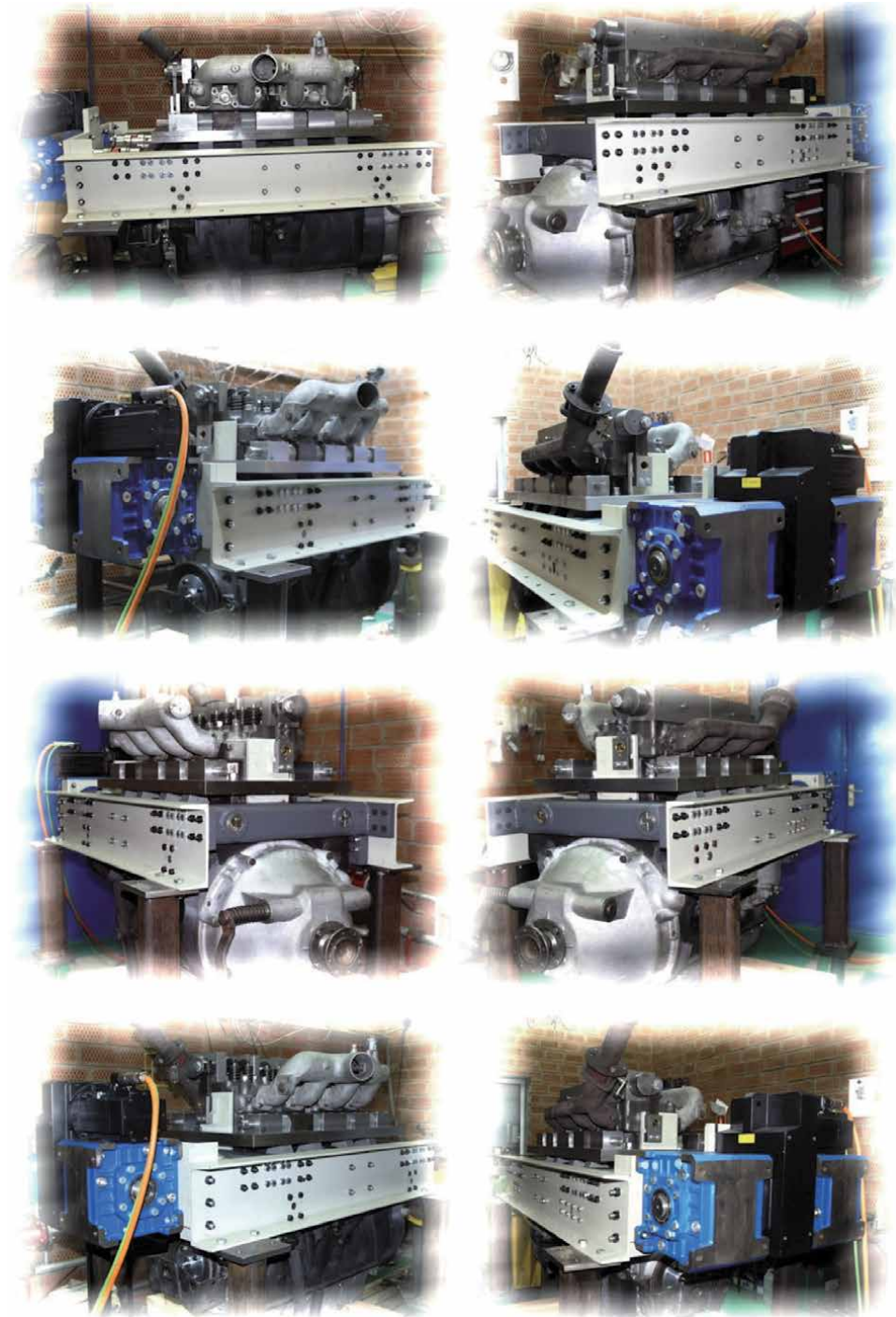
Figure 14. View of the complete VCR engine during functional tests.
