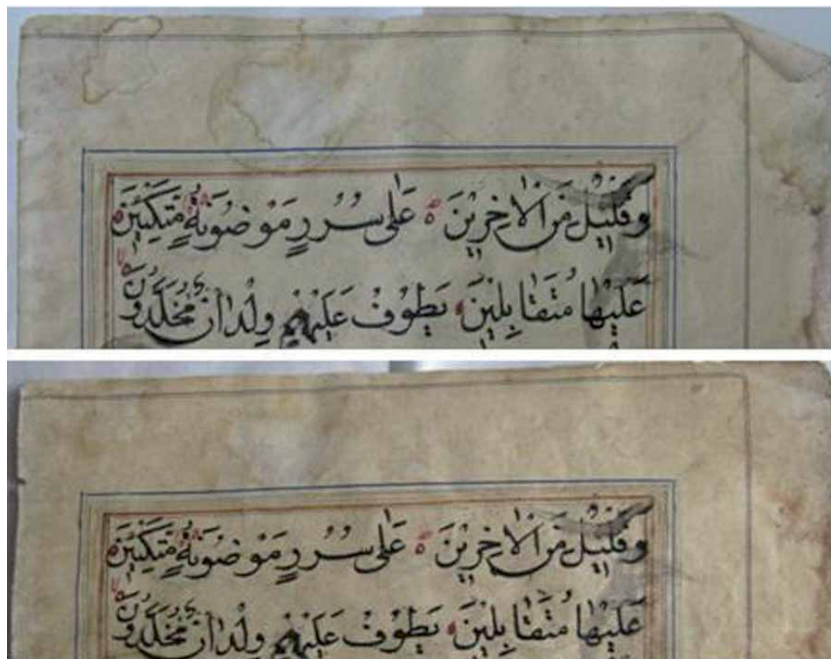
Figure 3. The visual aspect of old paper sample untreated (upper) and coated with nanocomposite ZnO NPs –Klucel (bottom) [44].
