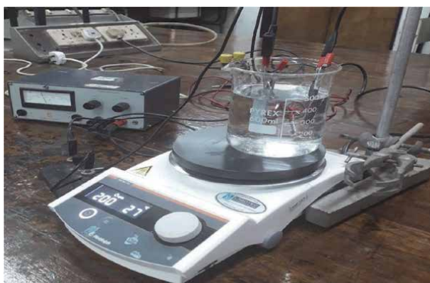
Figure 4. Plate showing the experimental setup for anodizing zinc metal.
