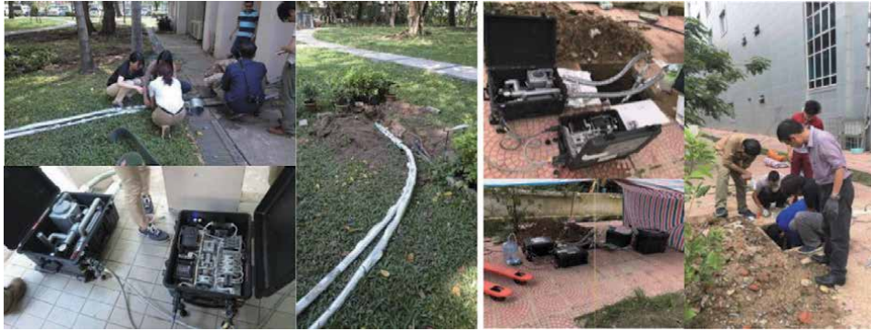
Figure 1. TRT measurement at the GSHP sites: Chulalongkorn University, Bangkok (left) and VIGMR, Hanoi (right).
