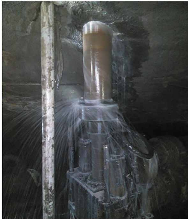
Figure 29. Overcoring test at KTK 8 Incline.
