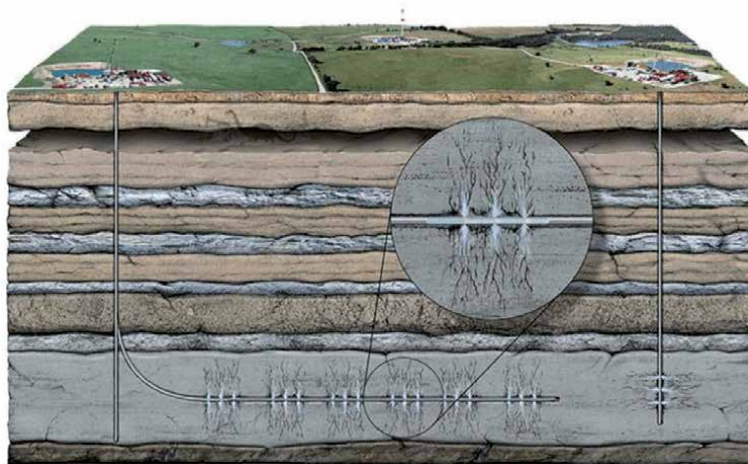
Figure 1. Sketch map of vertical well and horizontal well fracturing [4].
