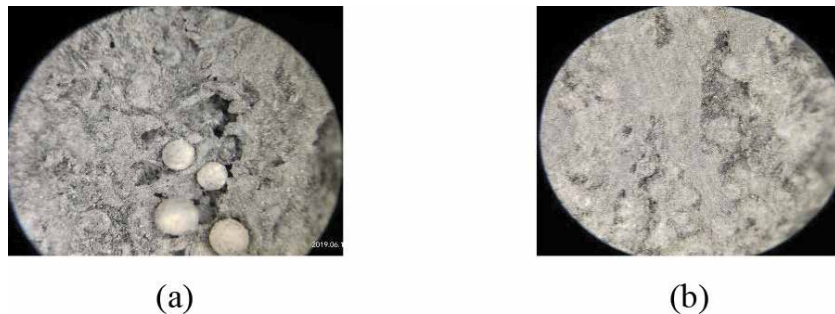
Figure 8. SEM images of proppant (20/40 mesh) embedment on the original core soaked in fracking fluid: (a) bottom of the core and (b) top of the core.
