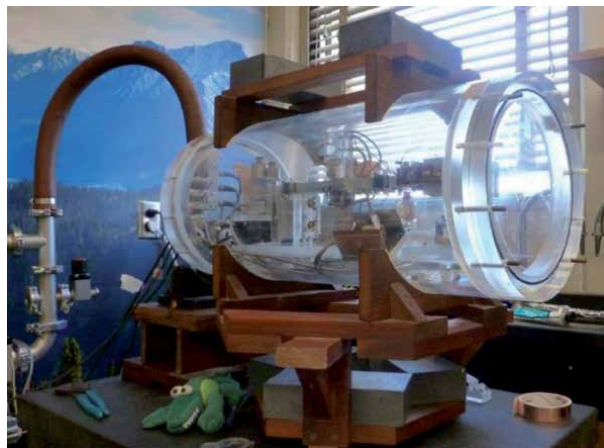
Figure 3. The torsion balance used in this work for small thrusts on its 500 pound granite vibration isolation table. The vacuum chamber is clear plastic, making careful examination of the operating conditions with a Polytech laser vibrometer easy.
