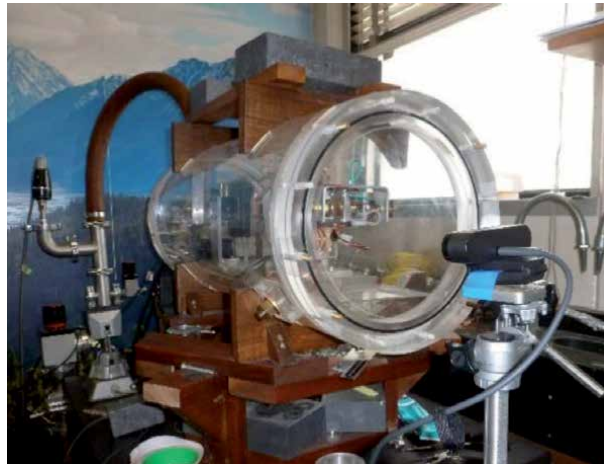
Figure 7. A sledge mounted device on hardware on the torsion balance in the clear plastic vacuum chamber.
