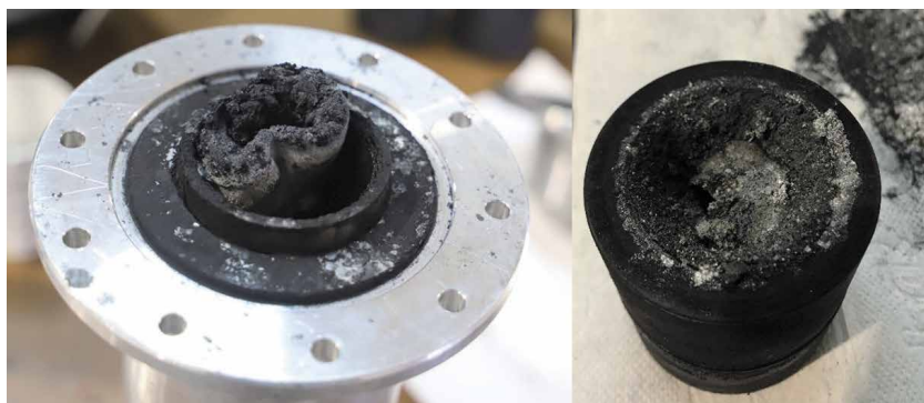
Figure 13. Oxide formation after the motor experiment.
