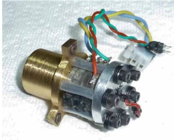
Figure 5. A bare device of the sledge design. The cap is 4.5 mm thick and 28.6 mm in diameter. High strength steel 4–40 cap screws provide the stack preload. Electrical connections are positioned to minimize drag on the motion of the parts.
