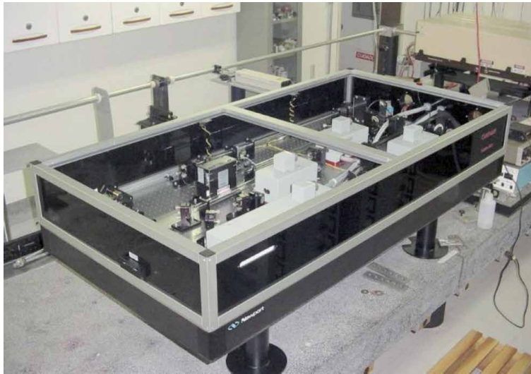
Figure 3. Photo presenting the continuum narrowband tunable laser for Na concentration and Mesopause temperatures. It operated at São José dos Campos measuring mesopause temperature from 2007 to 2009 and Na concentration from 2006 to 2016. This photo was taken by Barclay R. Clemesha (in memoriam).
