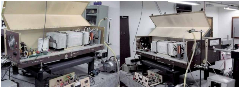
Figure 5. Photos showing the candela laser system assembled at INPE São José dos Campos in 1993. This system operated between 1993 and 2006—Photos taken by B. R. Clemesha (in memoriam).
