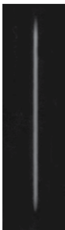
Fig. 9. Black and white silver halide photograph of the near-Gaussian emission beam, from the interferometric emitter (DICOS), recorder under nanosecond pulsed excitation at \sim 10 kV per pulse. The corresponding excitation current density is \sim 190 A/cm 2 (from Duarte (2008)).
