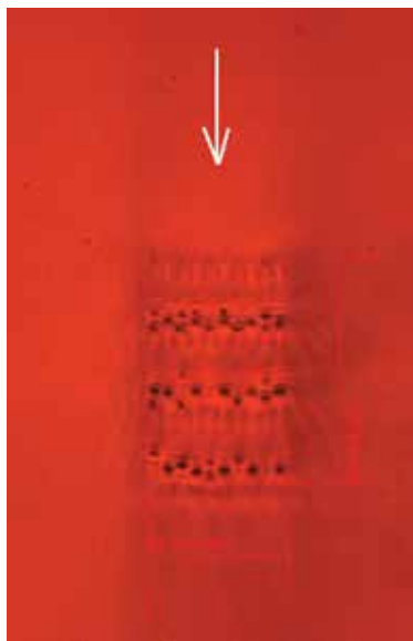
Fig. 2. End view of a waveguide written by Ti:Sapphire oscillator operating at 11-MHz rep rate. The arrow indicates direction of the femtosecond beam.
